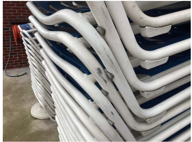
Frame finish deterioration
